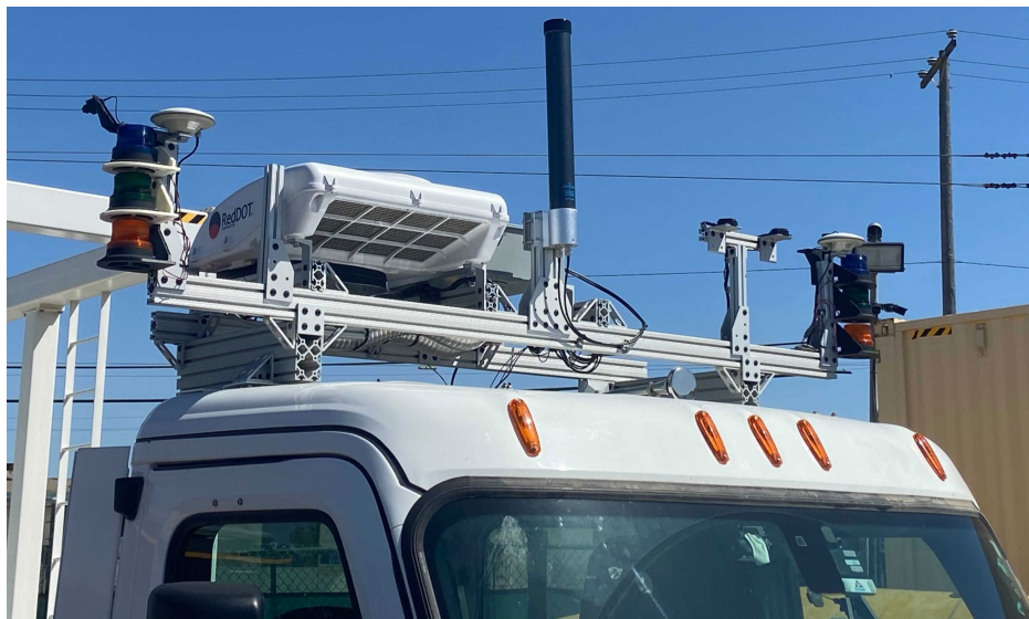
Figure 2. Photo. Longhorn mounted on roof rack.
